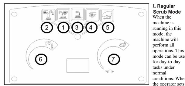
1. Regular **Scrub Mode** When the machine is running in this mode, the machine will perform all operations. This mode can be used for day-to-day tasks under normal conditions. When
